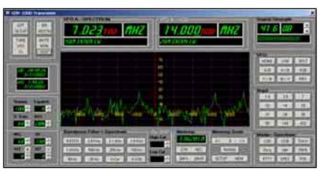
Fig 19—SDR-1000 front-panel display.
